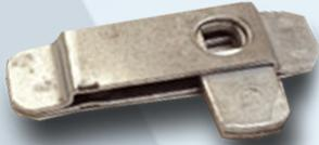
This lock is the standard Access Panel lock. The lock has a mild steel casing with a spring mechanism, and is operated with a Square Key.
