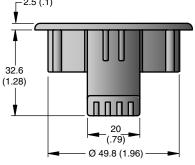
Align latch with frame, secure with mounting cup and self tapping screws (supplied with all parts).
