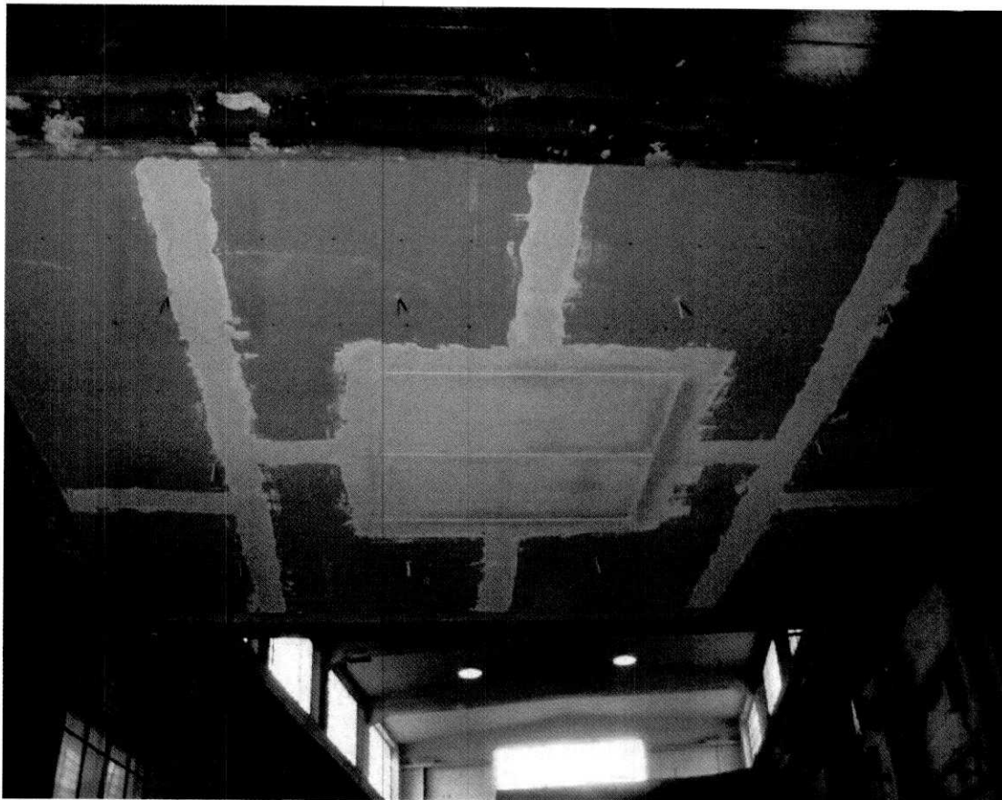
Plate 1 Exposed face of specimen before test showing furnace thermocouple locations
