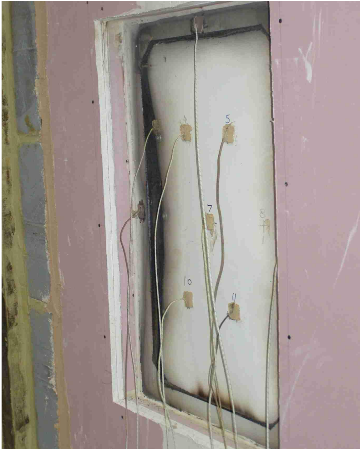
Photo 9 Unexposed face of access panel after test
