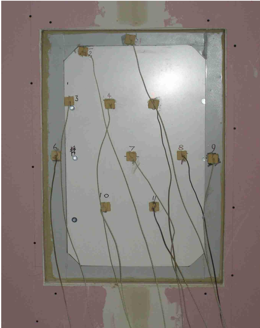
Photo 8 Unexposed face of access panel before test
