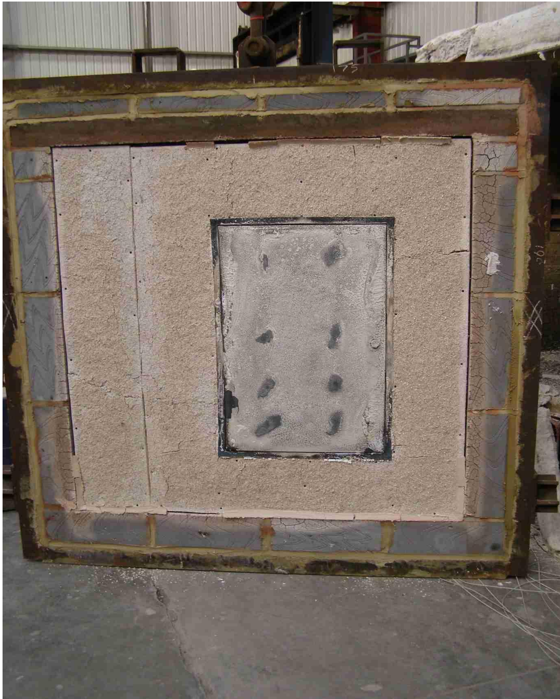
Photo 10 Exposed face of access panel after test
