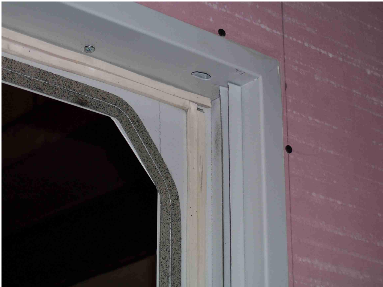
Photo 2 Access panel frame before test
