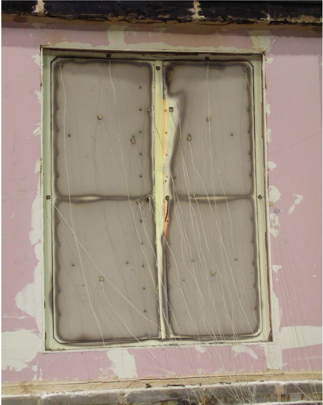
Unexposed face of specimen at end of test.
