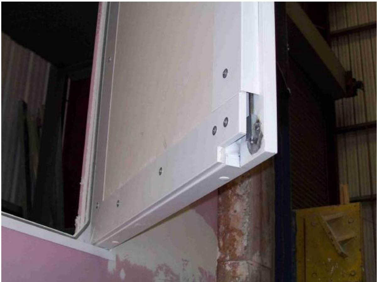
Photo 1 Open access panel active leaf before test
