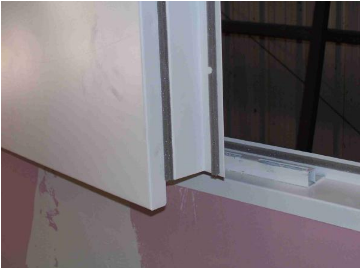
Photo 5 Base of passive leaf of access panel before test
