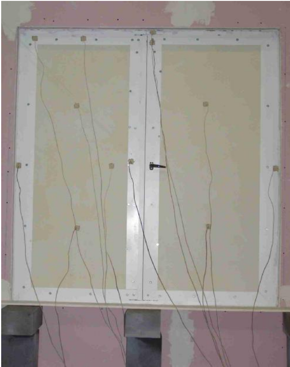
Photo 8 Unexposed face of access panel before test
