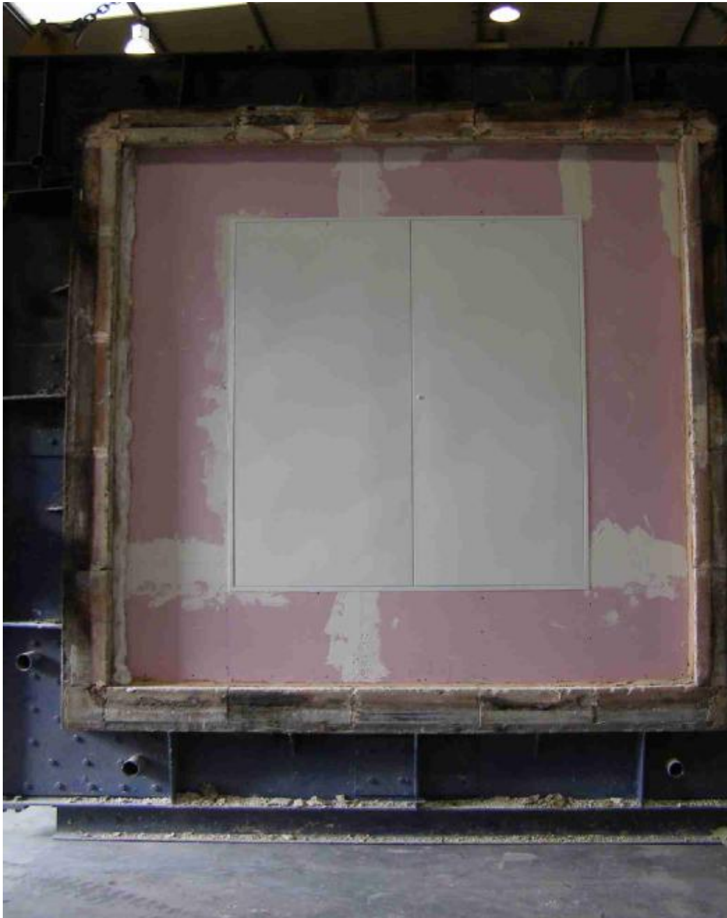
Photo 7 Exposed face of test construction before test
