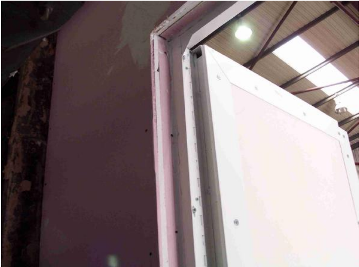
Photo 2 Open access panel active leaf before test
