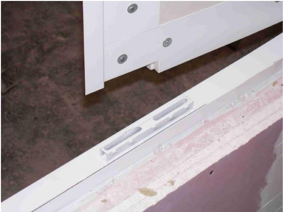
Photo 4 Base of passive leaf of access panel before test
