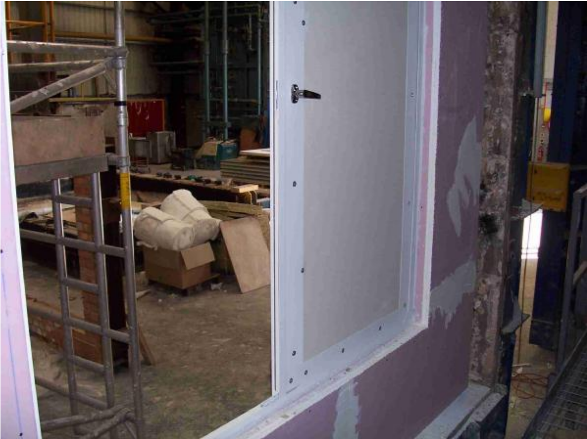
Photo 3 Access panel before test
