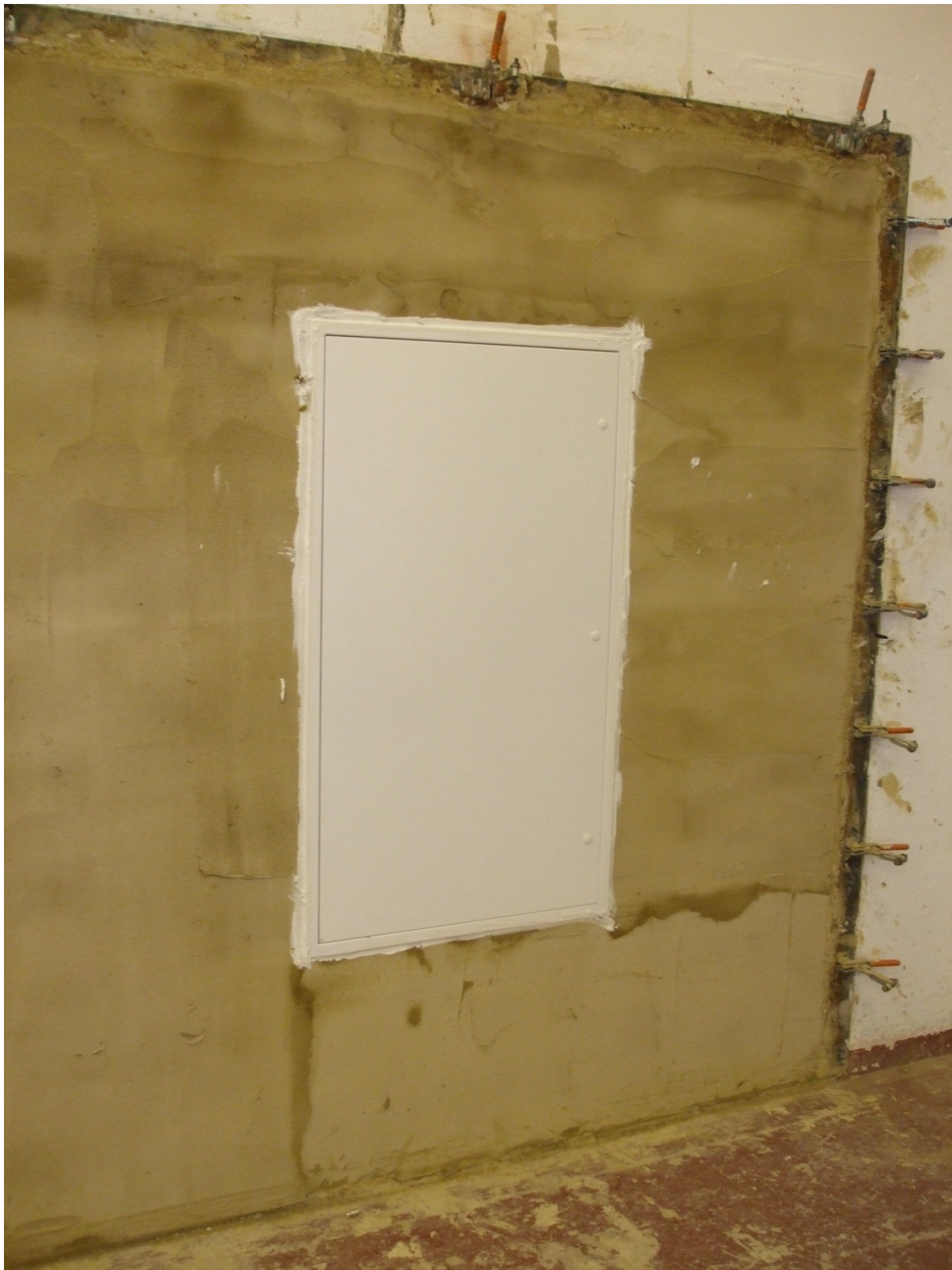
Photograph 1 – Access Hatch installed in Test Aperture
