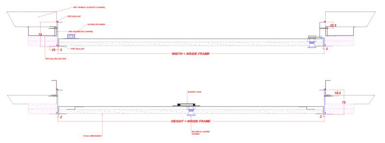
This panel is designed to fit into a structural membrane of a joint-less plasterboard ceiling system. It is manufactured with a Beaded frame for tape and jointing / skim-coat plastering. The panel has a Plasterboard faced door for tape and jointing / skim-coat plastering. The panels door leaf is locked in place via a Budget Lock as standard other lock options are available upon request. The Panel is Powder Coated RAL 9010 30% Gloss. Other colours available upon request.
