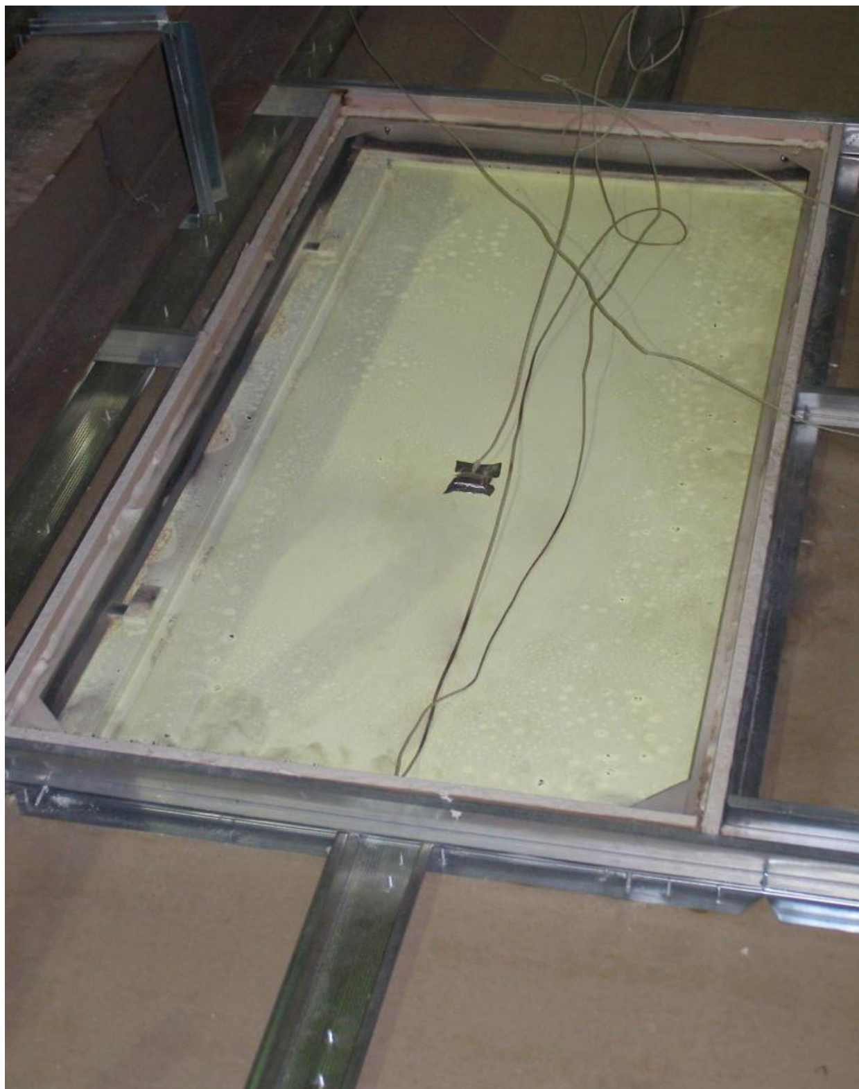
Unexposed face of ceiling showing MTFD access panel after 30 minutes.
