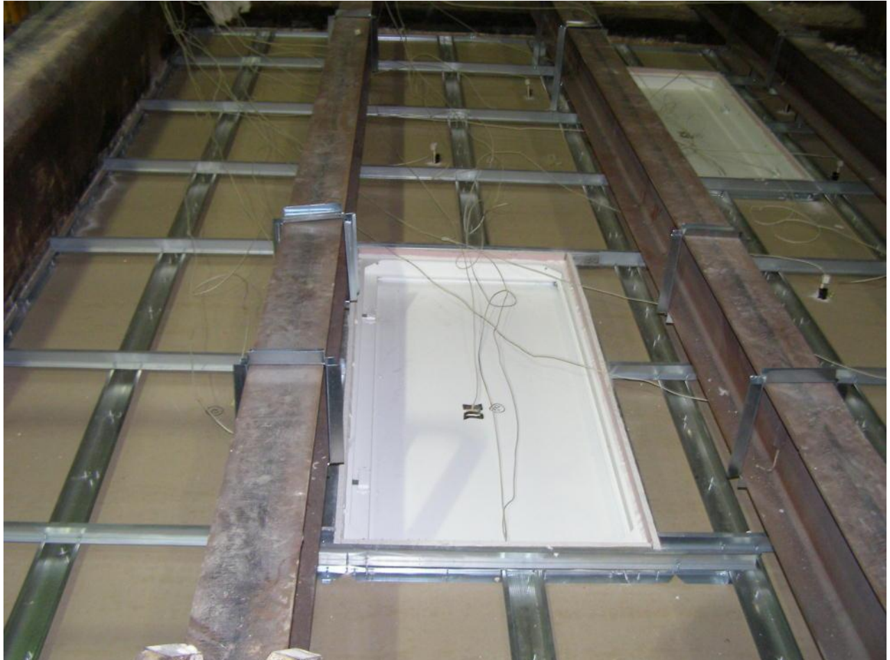
Unexposed face of ceiling showing MTFB access panel before test.
