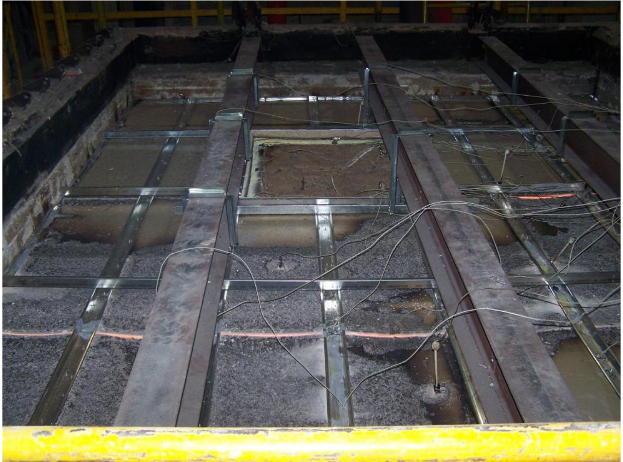
Unexposed face at end of test.
