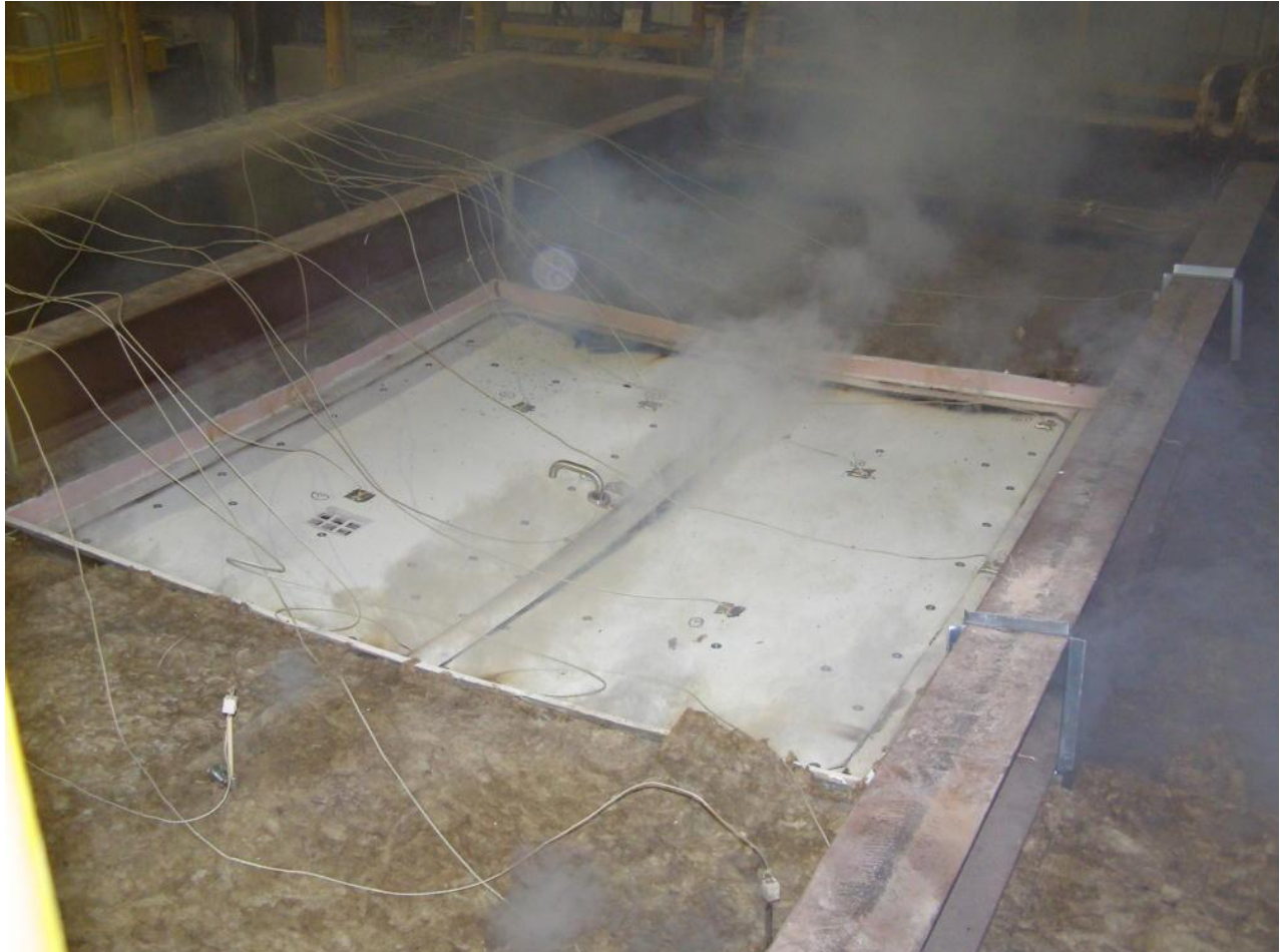
Unexposed face of specimen after 30 minutes.
